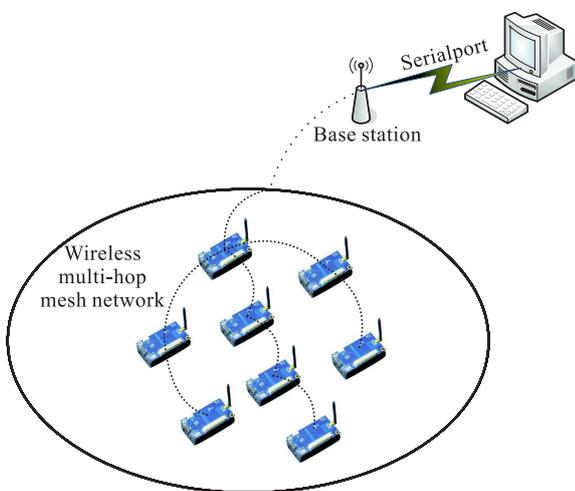
Fig. 2 Data acquisition network topology.
