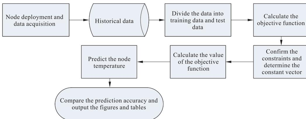
Fig. 1 Flowchart for predicting the temperatures.
