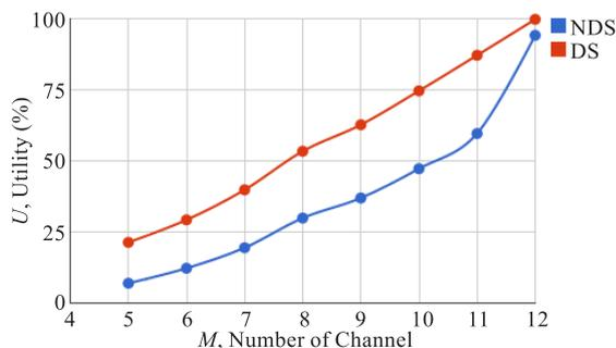
**Fig. 2** Performance of system of CR networks ( $N=12$ ) with multiple channel requirement. NDS - no deference structure, DS - with deference structure.
