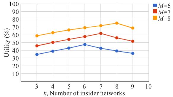
**Fig. 6 Performance of deference structure community of size  $k$  with varying  $M$ , number of spectrum bands. The optimal  $k$  corresponds to the peak of the curve.**
