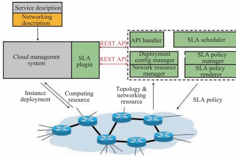
Fig. 2 Overall architecture of SLA subsystem.
