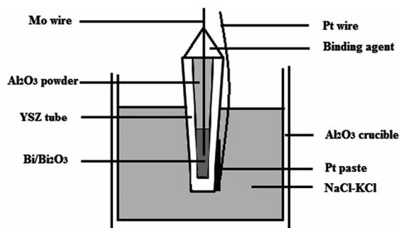
**Fig. 1** Setup used to determine the oxygen content of molten NaCl–KCl.
