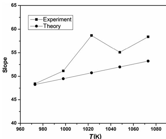
Fig. 3 Deviation between measured and theoretical slopes of EMF vs.  $\lg p_{O_2}$  plots as a function of temperature.
