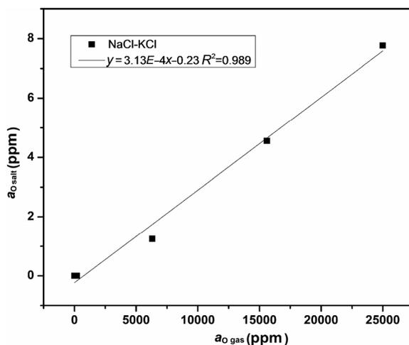
Fig. 4 Oxygen content ( $a_{O \text{ salt}}$ ) of molten NaCl–KCl as a function of  $O_2$  partial pressure ( $a_{O \text{ gas}}$ ) in covering gases.
