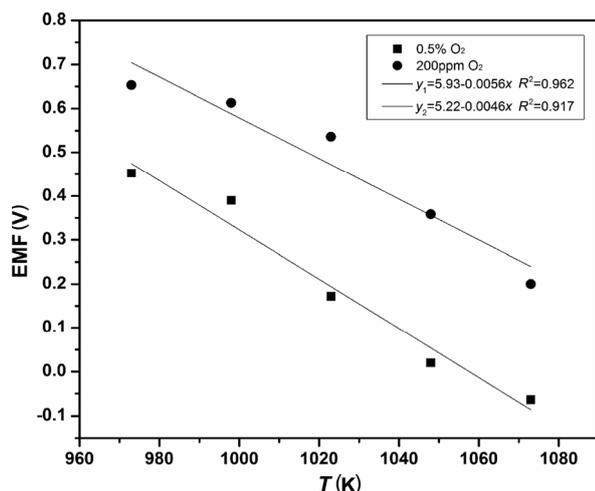
**Fig. 5** Dependence of EMF on temperature in molten NaCl–KCl.
