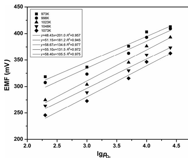
**Fig. 2** Results of accuracy measurements performed using the Bi/Bi<sub>2</sub>O<sub>3</sub> sensor at variable temperatures.
