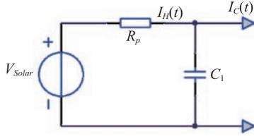
**Fig. 8** Equivalent energy harvesting circuit of IEA.
