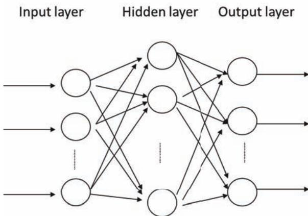
**Fig. 3 Structure of the artificial neural network model.**
