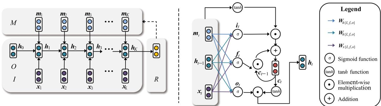
Fig. 2 Architecture (left) of FBMN and the detailed schematic (right) for hidden vector generation.
