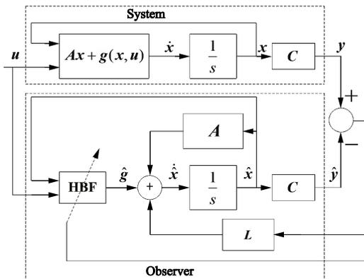
**Fig. 1** Observer model for nonlinear systems based on neural networks.
