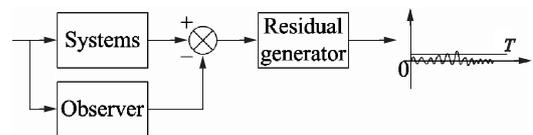
**Fig. 2** Detection principle.
