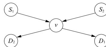
Fig. 1 X-type coding structures for COPE.
